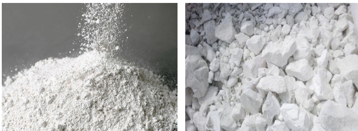
Figure 7: Hydrated lime is a free-flowing white powder (left). Clumps or cakes would indicate old lime (right)
