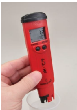
Figure 12: A common portable pH meter that can be used to monitor pH (source: Hanna Instruments, Inc.).
